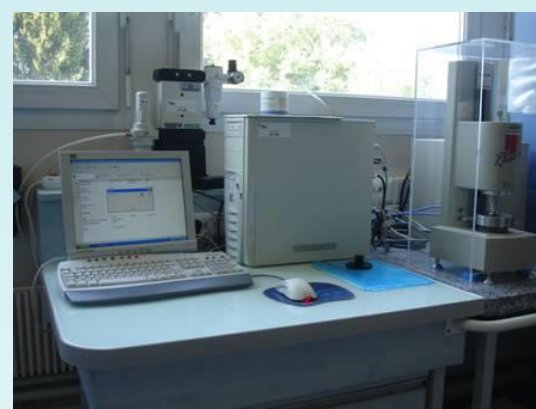
Rheometer: AR 1000 from TA Instruments
